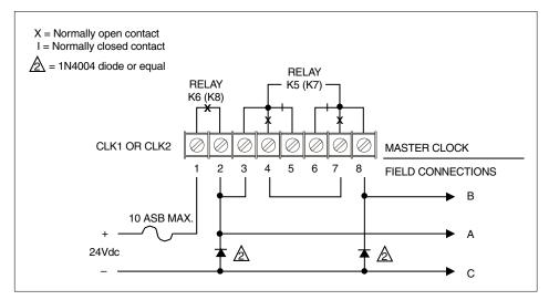
Figure B-23 Three-Wire Minute Impulse (44th Minute)
